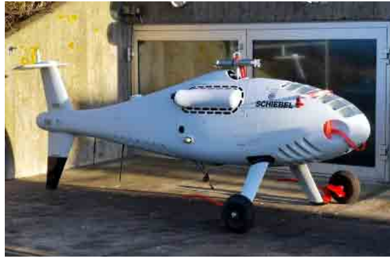
The drone being employed in 2020 to measure sulfur content in emissions
